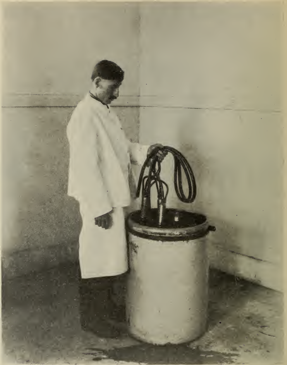
FIG. 9.—Incorrect method of immersion. When tubes are placed in solution folded up as above, the solution cannot come in contact with the whole of inner surface owing to pockets of air remaining in the tubes.
